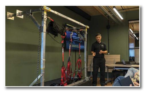
Stronghold requires no drilling, no fixings, and causes no damage to the property. Designed to be assembled quickly inside the building, it creates secure anchor points for harnesses and allows engineers to move freely and safely at height.
